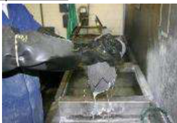
Step 2: Wash pre-filter sock thoroughly. Rinse through thoroughly in clean water and squeeze as much water out as possible. Leave to dry thoroughly before replacing.
