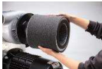
Step 2: Withdraw the filter end-plate and filter assembly over the fixing stud.
