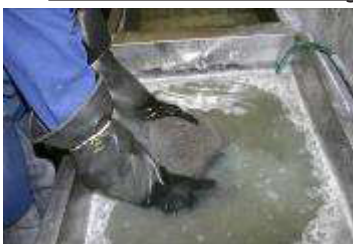
Step 1: Place the pre-filter sock in warm water, preferably with a low foaming detergent.
