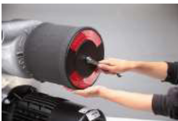
Step 1: Remove pre-filter element by releasing the security nut and washer. Use a 17mm AF spanner.
