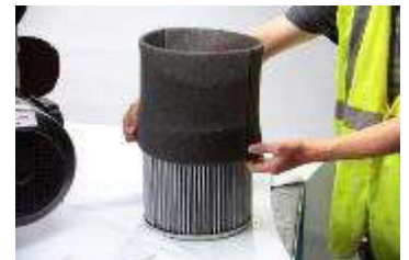
Step 3: Remove the pre-filter sock from the main filter element.
