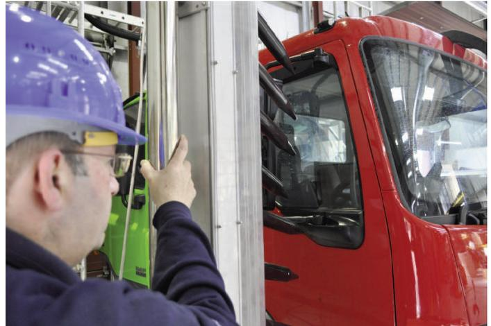
Testing ACI Reciprocator Nozzles on Truck Cabins
