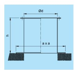
The roof upstand is used for elevated installation of roof fans, such as for compensation of snow heights or insulations.
