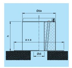
The sound-absorbing upstand is used for damping the sound power radiated into the suction line.
