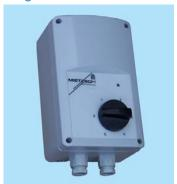
The transformer induced 5-stage control unit RE is used for manual speed control of fans with external rotor motor. Contrary to electronic voltage setting (such as phase angle control, frequency conversion), the sinusoidal control voltage does not lead to additional motor noise or feedback to the mains.
