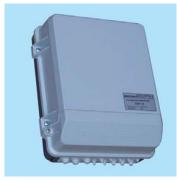
The timer-control ZSK is used for the speed control of fans with external rotor motor. The sinusoidal control voltage does not lead to additional motor noise or feedback to the mains
