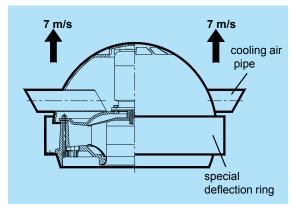
The special version LAB leads to the outlet speed of 7 m/sec. if the following condition is met:
