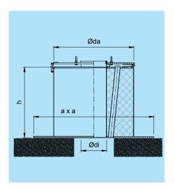
The sound-absorbing upstand is used for damping the sound power radiated into the suction line.
