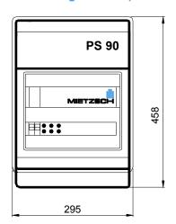
The pole changer of type PS 90 is a compact solution for the control of fans with polechanging motors.
