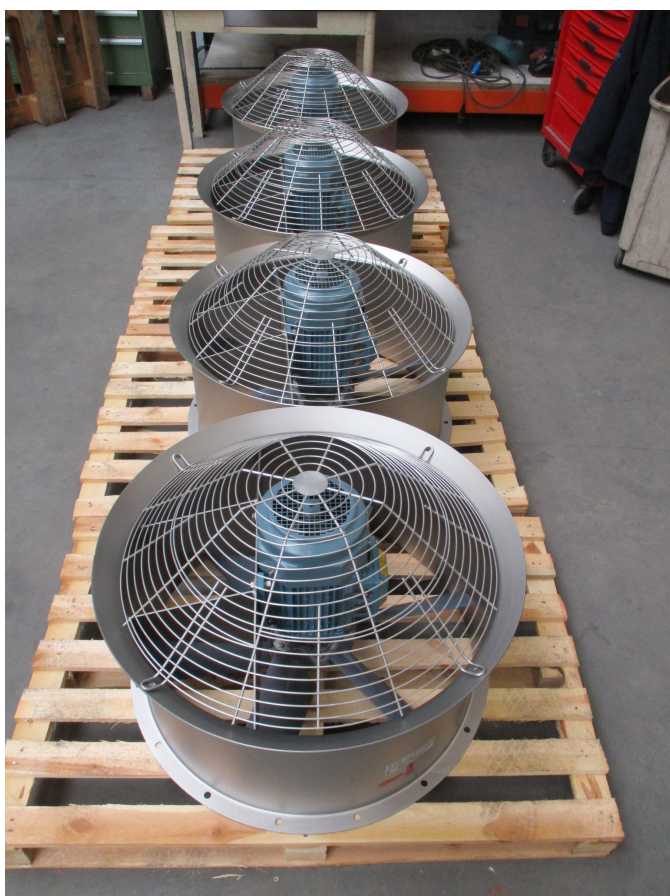
Type : AVKEX 710/6P/6-6/P5Z/PACAS/L/50°/A10° Motor : 1,5kW 3x400V 50Hz EexnA II T3 Atex : II 3G c II BT3 Q= 17.000 m 3 /h, Hstat= 79 Pa at 29°C
