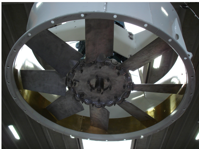
Type : AVKEX 1000/4/8C/10° Motor : 15kW 3x400V 50Hz EexnA II T3 Atex : II 3G c II BT3 Q= 40.000 m 3 /h, Htot= 650 Pa at 50°C
